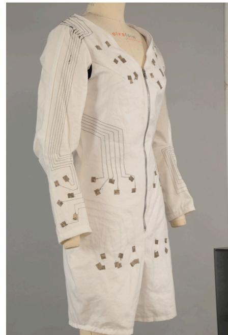
Figure 1. Reconfigurable e-textiles garment, showing swatch locations
