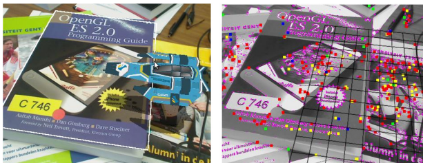
Figure 2. The application tracks feature points (right) to enable the overlay of 3D objects (left).
