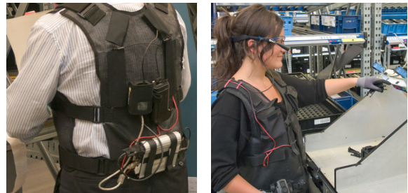
(a) Back: wearable computer, (b) Front: rugged mouse and battery status LED antennas
