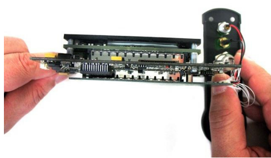
Image 3 – teXXmo ONE three-layer architecture
