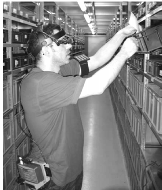
Fig. 7: Prototypal order picking with a head mounted display
