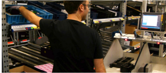
(b) After pick detection, the light turns green and red lights on the pick-cart indicates where to put the items (and how many items are needed in total)
